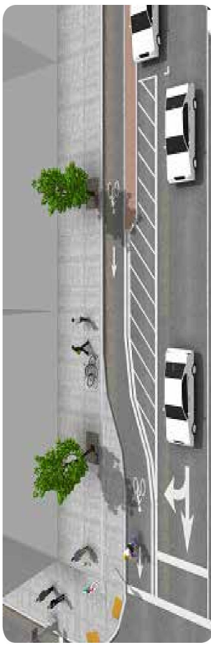
Example of a cycle track bending in towards the roadway and parking restrictions when approaching an intersection
