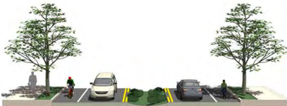
Figure 3-E. Collector 3-Lane Cross Section
