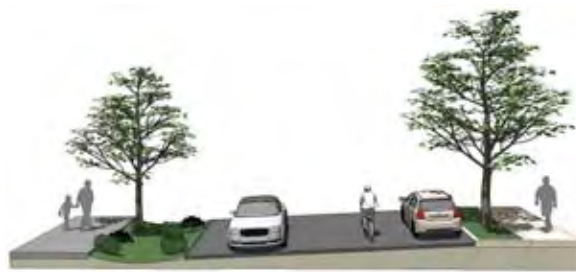
Figure 3-I. Hillside Local Street With Stormwater Swale
