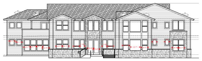
The east ground floor facade measures 169' 2 %" in length. 169' 2 %" x .3 = 50.7'. The east ground floor facade requires 50.7' of windows between 3.5 feet and six feet from the ground. The applicant has proposed 41.5' of windows (measuring glass only). Based on this measurement, 9.2' of additional windows is required on the east ground floor front facade. Ground floor facade (east or left side):
