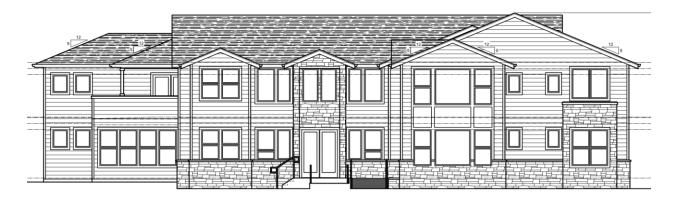
1. Street facing facades shall include additional design features. For every thirty feet of façade length, three of the following elements are required:
