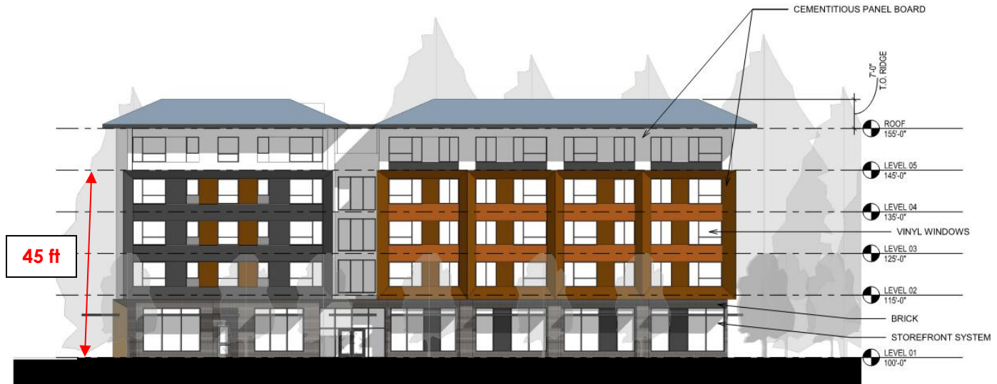
Figure 7: Building Elevation facing Llewellyn St
