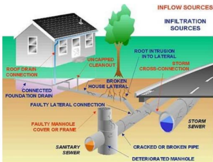
Figure 1: Typical sources of I/I in sanitary sewer systems. (Adapted from WE&RF, 2003)
