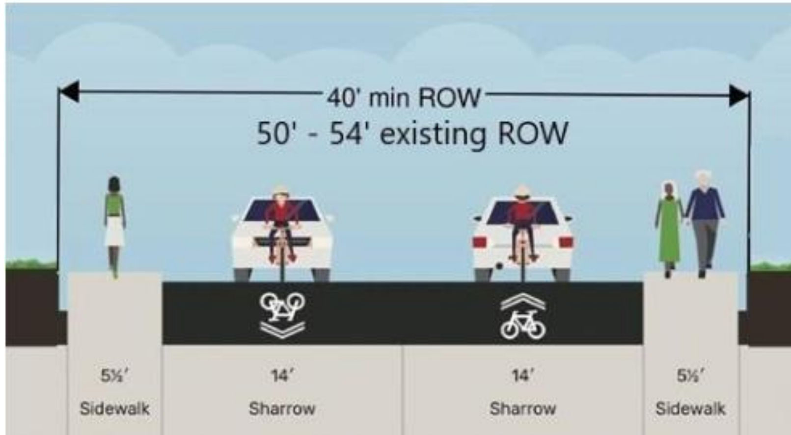
Figure 4-3: Apperson Street Cross Section
