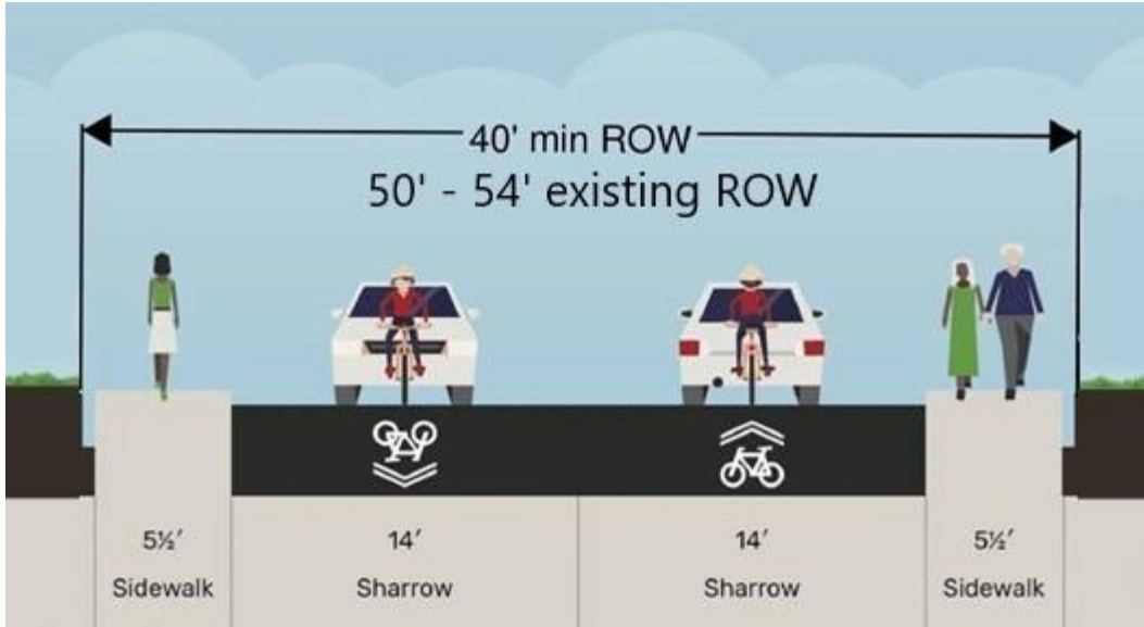
Figure 4-3: Apperson Street Cross Section
