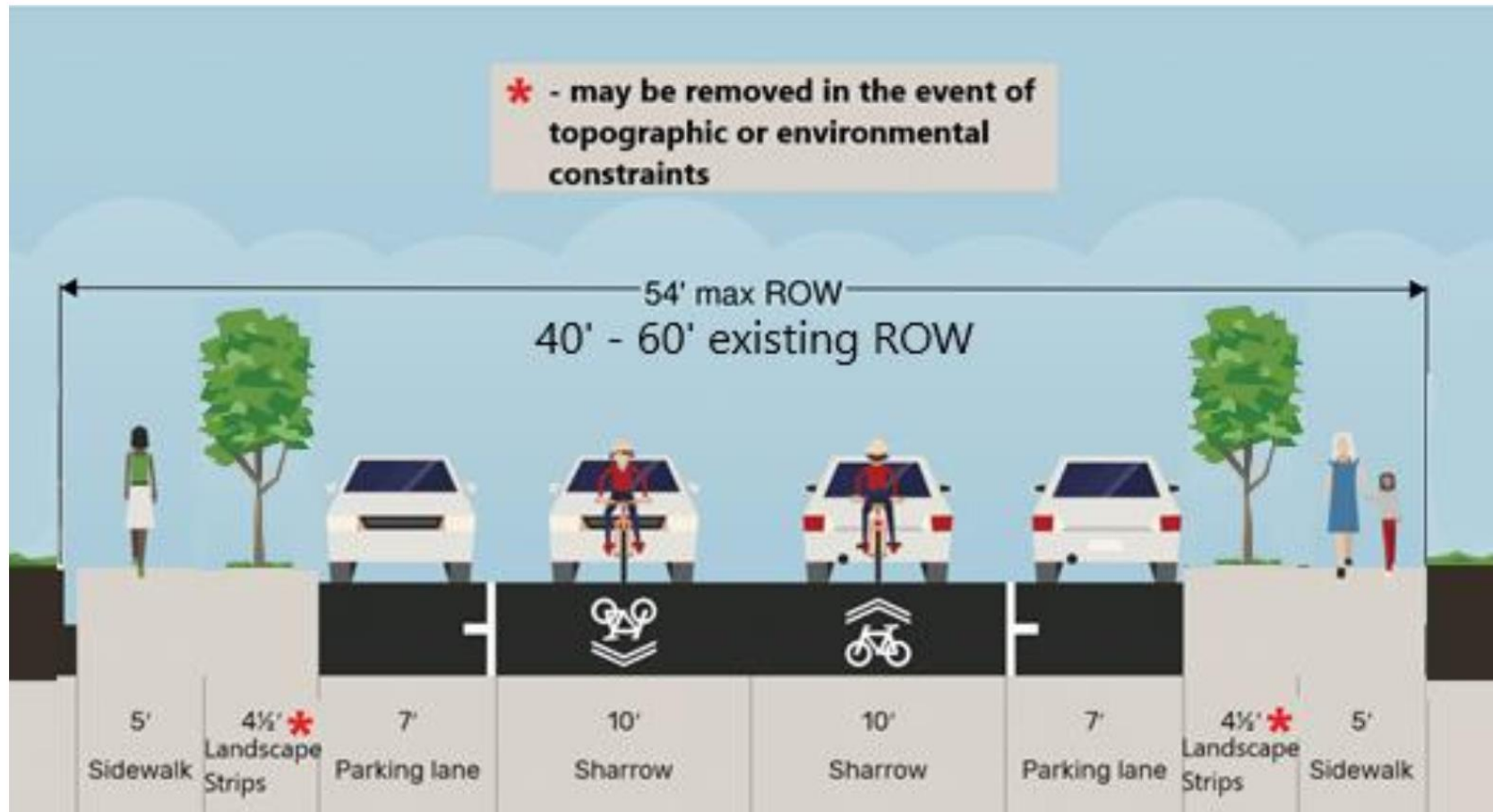
Figure 4-5: Hunter Street Cross Section
