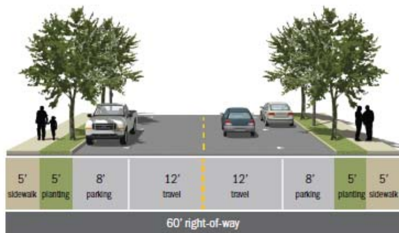
Figure X. Proposed Conceptual Cross-Section for Local Streets with a 60' right of way
