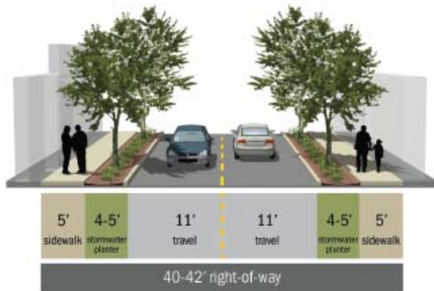
Figure X. Proposed Conceptual Cross-Section for Local Streets with a 40' right of way
