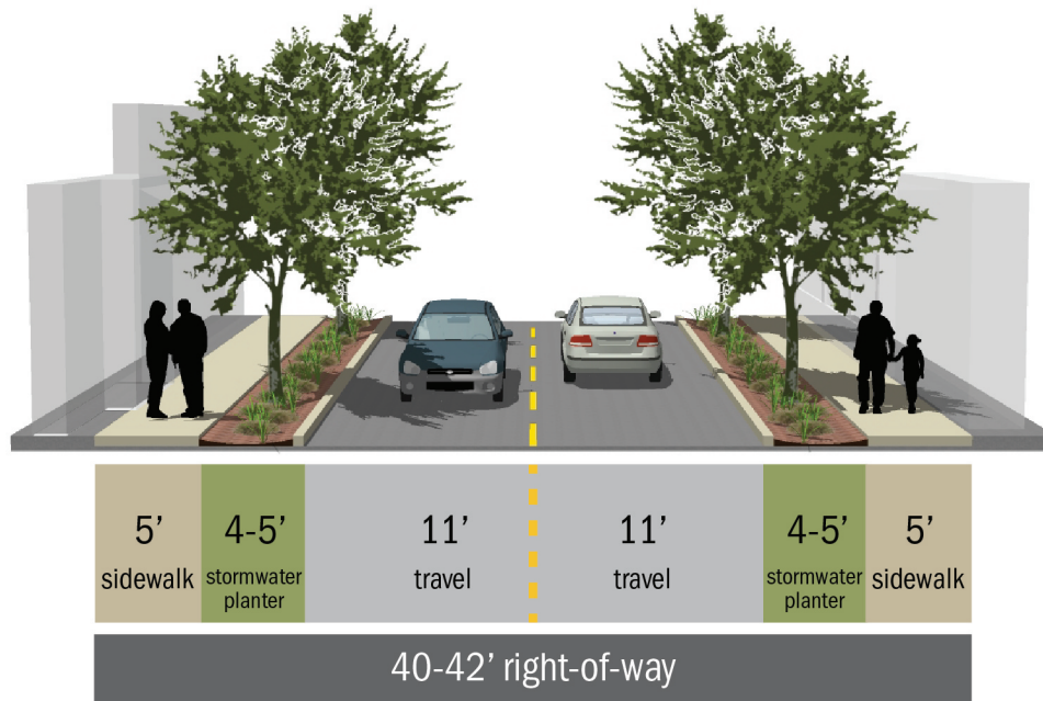
FIGURE 20: PROPOSED CONCEPTUAL CROSS-SECTION FOR LOCAL STREETS WITH A 40' RIGHT-OF-WAY
