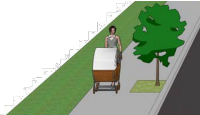
Option for Left Side of Street: widen sidewalk to 7.5 ft
