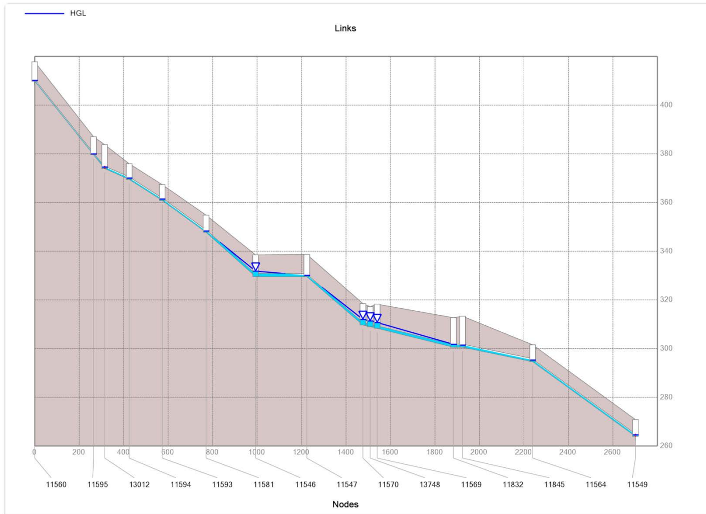
Figure 7. Linn Avenue sewer profile, 1- in 10-year storm event, pipes upsized
