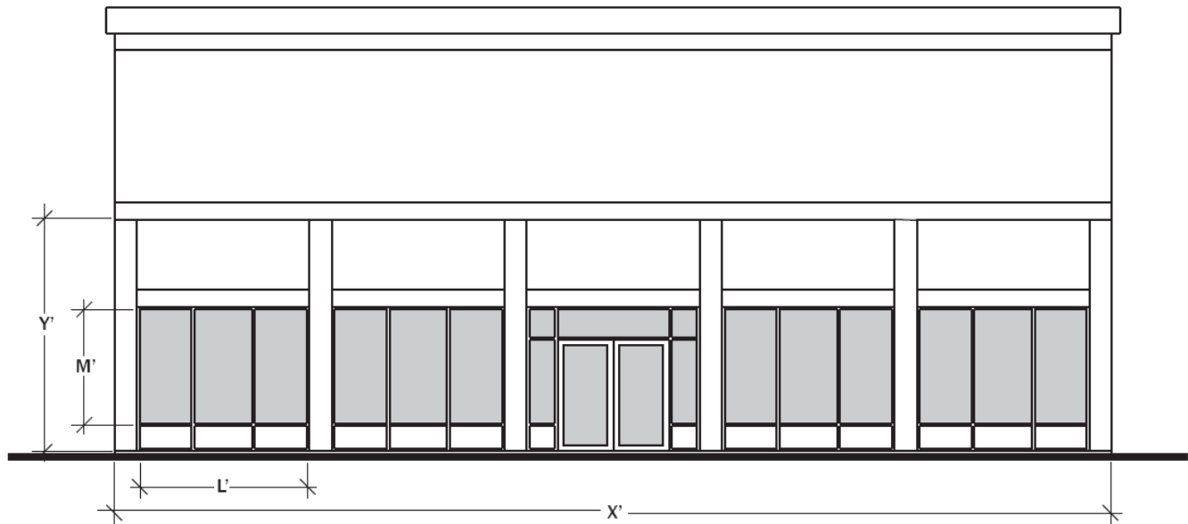
Figure 19.406-1 Ground Floor Windows and Doors
