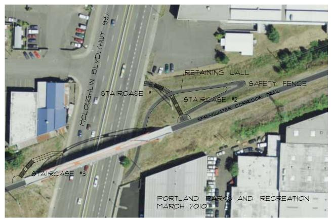
Figure C-1. Planned Improvements from Springwater Corridor to Light Rail Station
