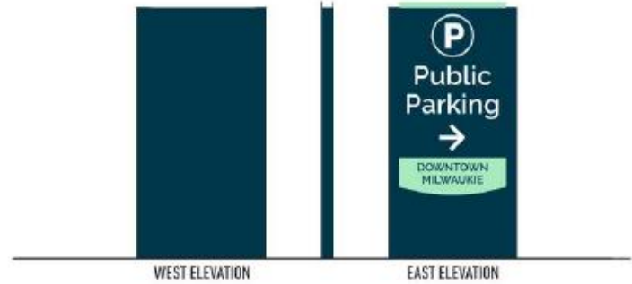
A2 | S/F POST AND PANEL SIGN - DETAILS - 8 SQ. FT. Scale: 1/2" = 1'-0"
